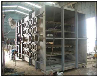
Water Quench Tank
