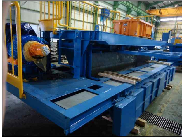
Reclaimer for Coal Silo
