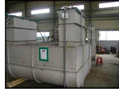
Mist Cooler Duct
