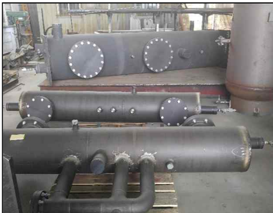
H2 Detraining Section
